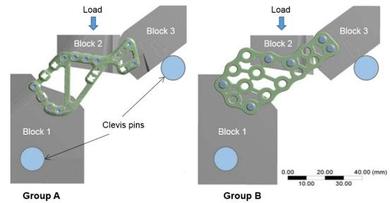
**FIGURE 1. Mechanical three-point test model.**
